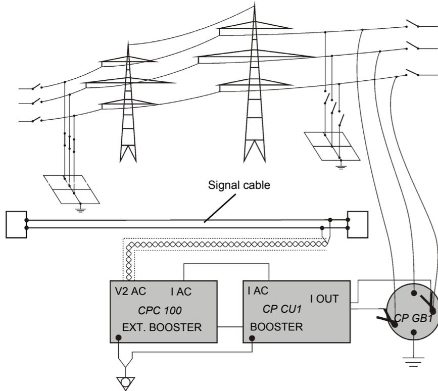
There are four measurements with different connections. For detailed information, refer to the template or the CP CU1 Reference Manual.
