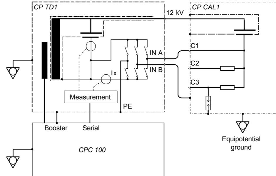
When using the CP CAL1 for calibration, we recommend to take C1 as reference and to select the calibration frequency in a range between 50 ... 200 Hz.
