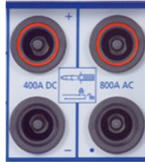
The counterpart of the high-current sockets are locking connectors. To lock these connectors safely, insert them carefully until you feel a "click" position. Now they are locked. Confirm this by trying to pull them out. This should not be possible now. To remove the locking connectors, unlock them by pushing them in completely first, and then pull them out.
