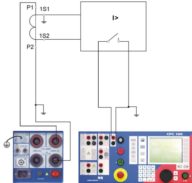
The CPC 100's **AC OUTPUT** feeds the ramped current signal into a CT, which is connected to an overcurrent relay. The overcurrent relay's trip contact is fed into the CPC 100's binary input **BinIn**, and acts there as a trigger signal.
