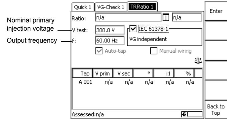
With the **IEC 61378-1** check box activated, the **CPC 100** carries out two standard-compliant measurements for each winding and calculates the transformer's turns ratio and phase shift. The measurement table displays the same values as for the standard **TRRatio** measurement. The magnetization current and phase angle will not be available in this mode.
