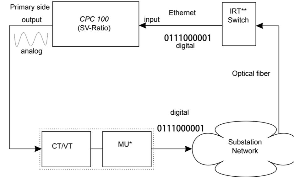
\* If the MU has an Ethernet output, no IRT switch is required.
