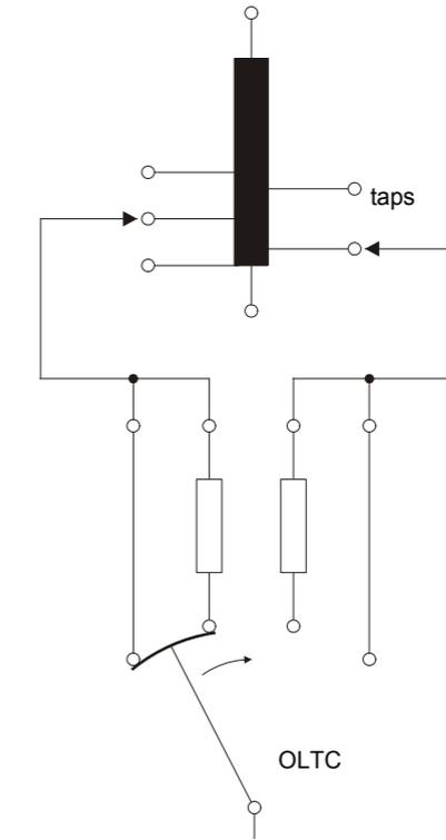
The **CPC 100** injects a constant current from the **6A DC** output into the power transformer and the current is led via the **I AC / DC** input for measurement. Alternatively, the current injected from the **400A DC** output is measured internally. From this current value and the voltage measured by the **V DC** input, the winding resistance is calculated.
