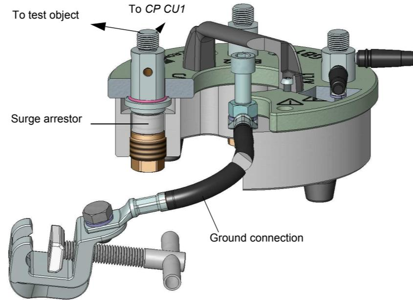
To short the phases, connect the line studs of the CP GB1 as shown below.
