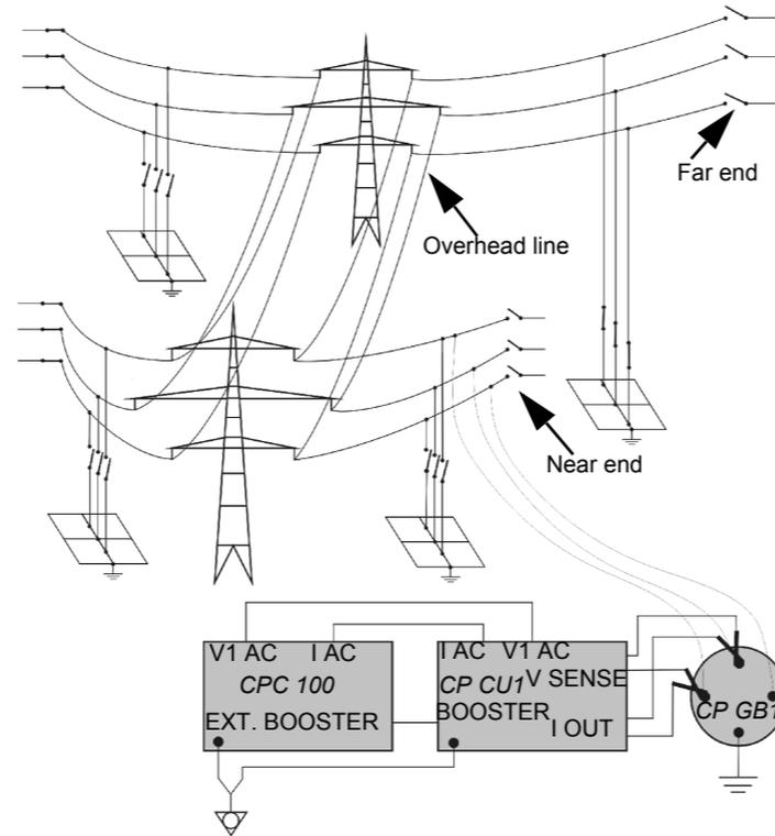
There are seven different measurement loops: A-B (shown here), A-C, B-C, A-G, B-G, C-G and ABC in parallel to ground (similar to the next figure).
