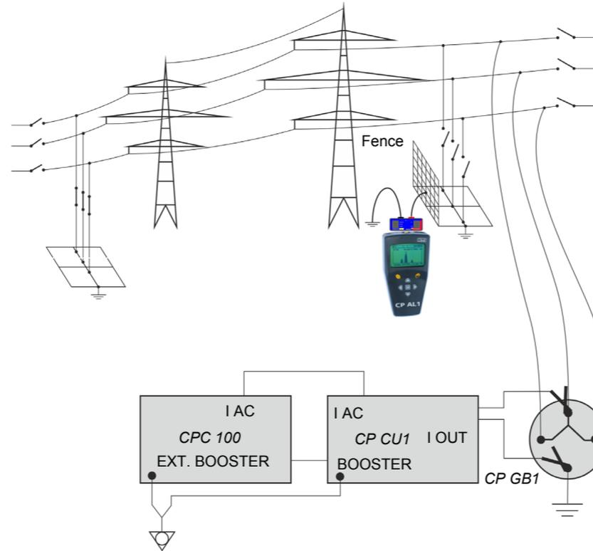
For the step and touch voltage measurements using the CP AL1 FFT voltmeter, refer to the CP 0502 Application Note.
