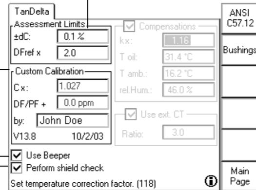
Selecting "Compensations" converts the actually measured dissipation or power factor to normalized values corresponding to an ambient temperature of 20 °C. In doing so, the values entered at "Compensations" represent the existing ambient condition.
