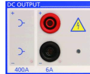
The message "Switch off in progress" notifies you that, after the *CPC 100* was switched off, the connected external inductance (i.e., the test object) still "feeds" voltage potential back into the **6A DC** or **400A DC** output.
