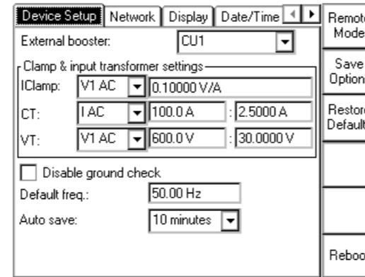
2. In the **External booster** combo box, select **CU 1**. The **CT** and **VT** settings are set according to the built-in current and voltage transformers automatically.
