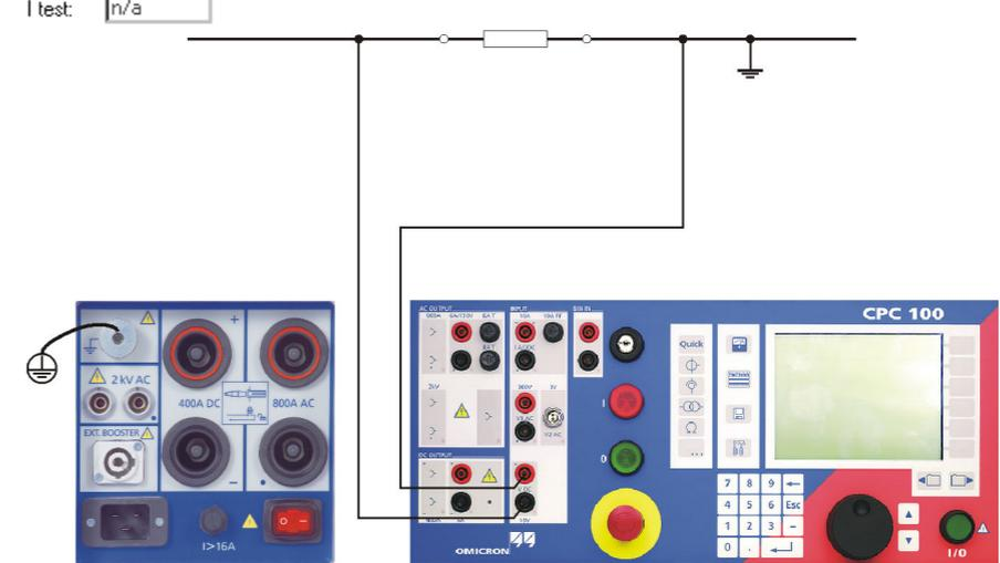
At this range, the DC input **V DC** outputs the current needed to measure the resistance.
