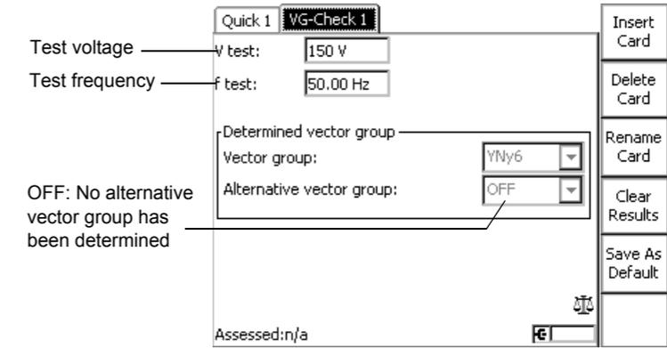
The **CPC 100** energizes the transformer's primary windings and measures the voltages on the secondary terminal. The optimized algorithm reduces the number of measurements. The vector group is determined according to the voltage distributions. In cases where the measurement results apply equally to two vector groups, an alternative group is provided.
