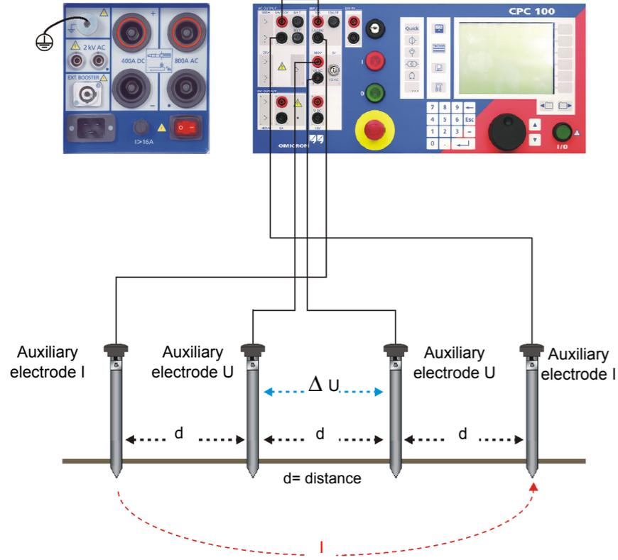
Calculating the soil resistivity:
