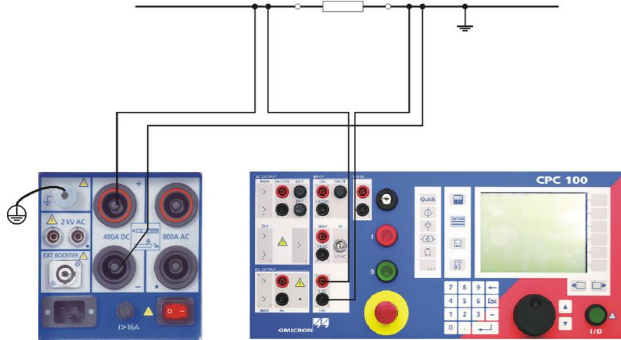
Inject current from the **400A DC** output to both sides of the test object. Input **V DC** measures the voltage drop, the software calculates the test object's resistance.
