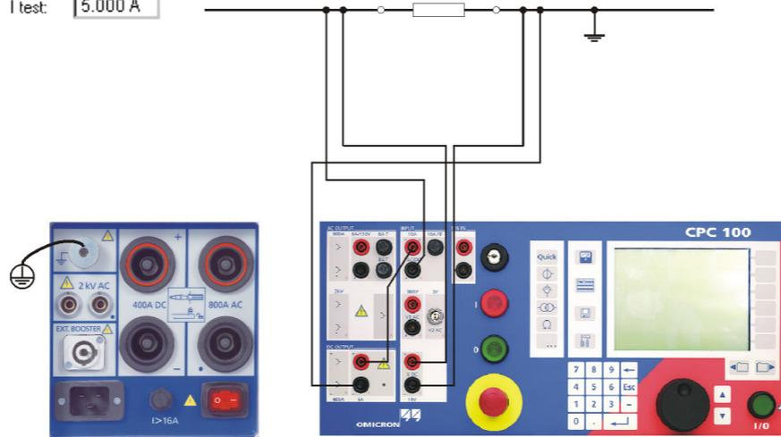
Inject current from the **6A DC** output to both sides of the test object. To measure this current, route it via the **I AC/DC** input as shown in the figure above. Input **V DC** measures the voltage drop, the software calculates the test object's resistance.
