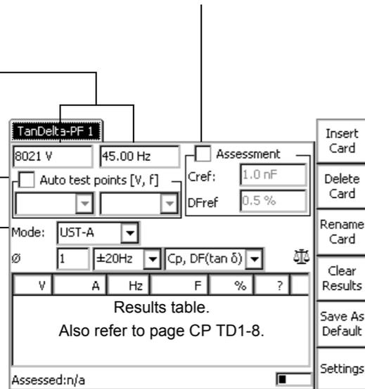
\*) **"Auto test points" cleared = manual measurement:** Applies the set test voltage and frequency to the *CP TD1*'s output. When the measurement is finished, its results are displayed in the results table.
