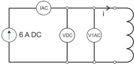
The **CPC 100 Demag** test card requires a **CP SB1** transformer switch box. The wiring is the same as for a standard resistance test plus a connection of the **V1** input to the switch box. Via the switch box, the **CPC 100** injects a constant current from the **6A DC** output into the power transformer. The current is led through the **I AC / DC** input for measurement.
