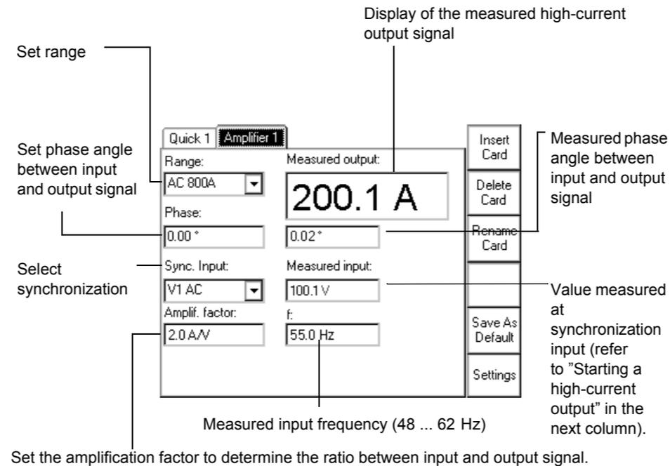
**Note:** The synchronization input is not automatically range-switching, it is fixed to its maximum value.
