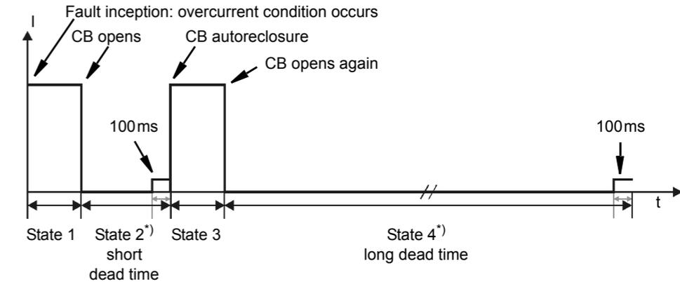
\*) State 2 and 4 incl. the additional 100 ms the CPC 100 adds to compensate for the debounce (see note above).
