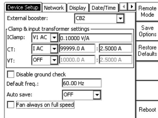
**Note:** If you select the *CP CB2* as external booster on the **Device Setup** tab in the **Options** menu, it will be saved as default value for new test cards. However, it is also possible to select the external booster individually on the test cards. The settings for already inserted test cards will only be changed if no test results are available yet.
