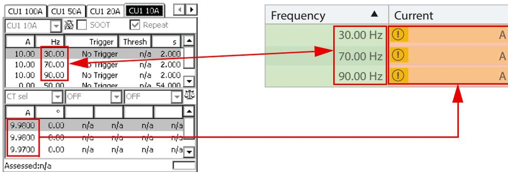
Figure 5-14: Enter the current readings under the **Settings and Conditions** section in *PTM*
