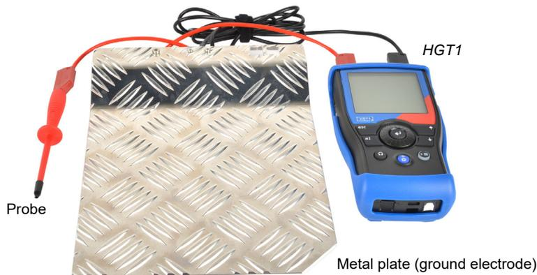
Figure 5-21: *HGT1* hardware setup according to EN 50522
