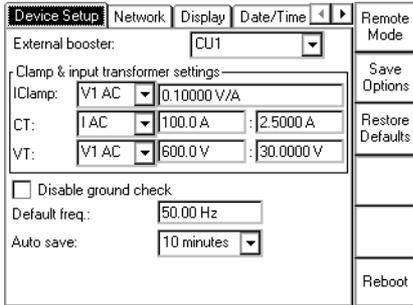
Figure 5-7: **Device Setup** tab of the *CPC 100 Options* menu
