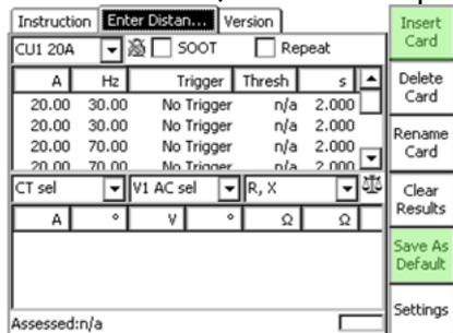
Figure 5-8: **Enter Distance** test card of the **Ground Impedance** template on the *CPC 100*
