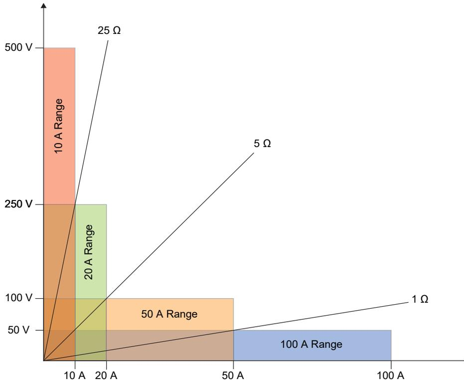
Figure 2-16: Load diagram of the *CP CU1*
