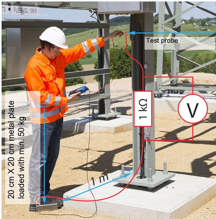
Figure 5-19: Touch voltage measurement according to EN 50522
