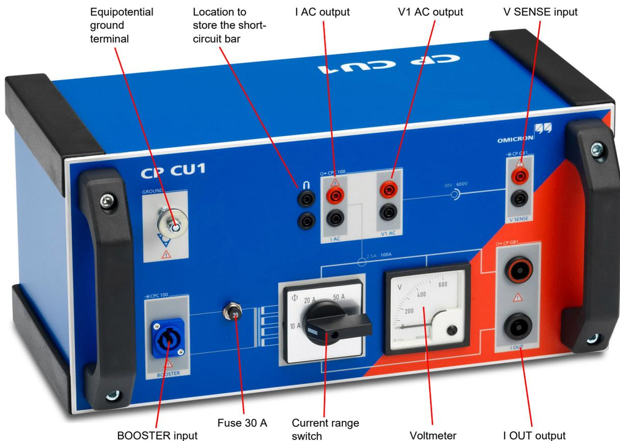
Figure 2-2: Front panel of the *CP CU1*
