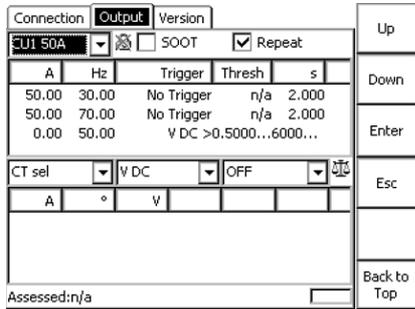
Figure 5-18: **Output** test card of the **Step&Touch using HGT1** template on the *CPC 100*, adapted for remote-controlled current injection
