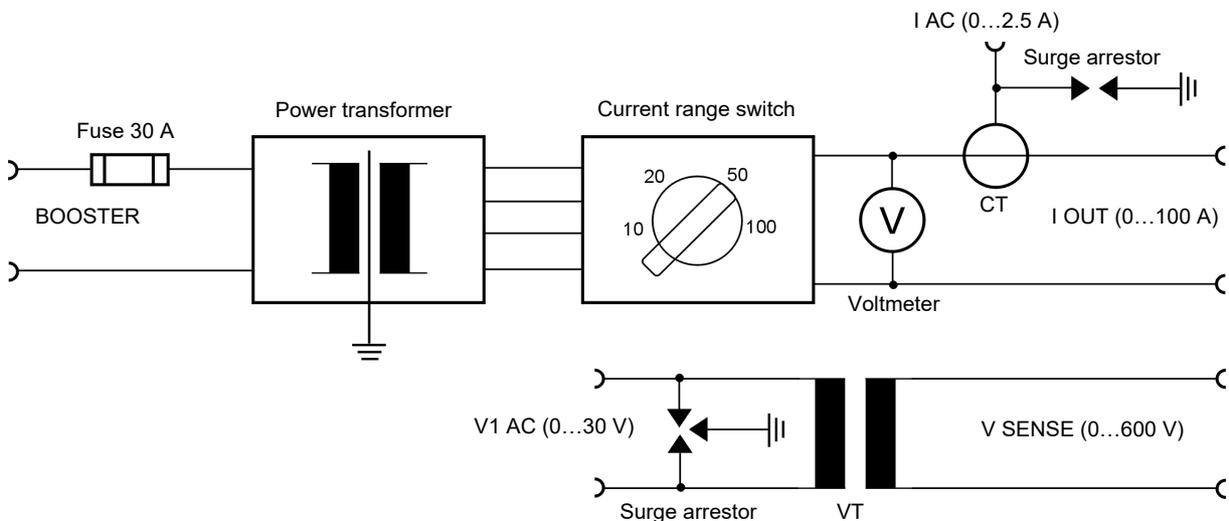
Figure 2-1: Circuit diagram of the *CP CU1*
