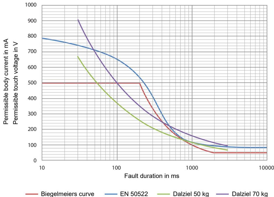
Figure 5-4: Permissible body currents from EN 50522 and IEEE 80
