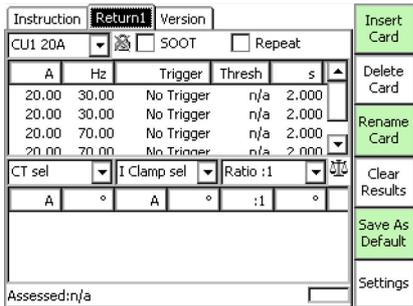
Figure 5-30: **Return1** test card of the **Reduction Factor** template on the *CPC 100*
