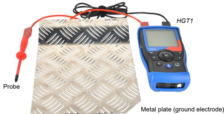
Figure 5-27: *HGT1* hardware setup according to EN 50522
