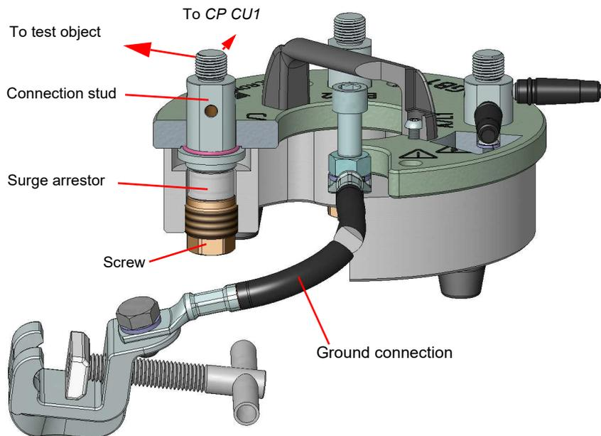
Figure 2-4: Cross-sectional view of the *CP GB1*
