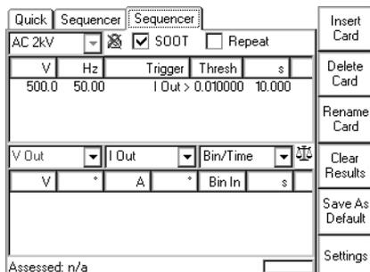
Figure 2-8: Setup of the sequencer test card for surge arrestor testing
