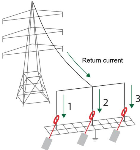
**Note:** The arrow marking on the connecting mechanism of the Rogowski coil (for closing it) needs to point in the direction of the current flow.
