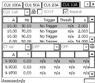
Figure 5-13: CU1 10 test card of the PTM template on the CPC 100
