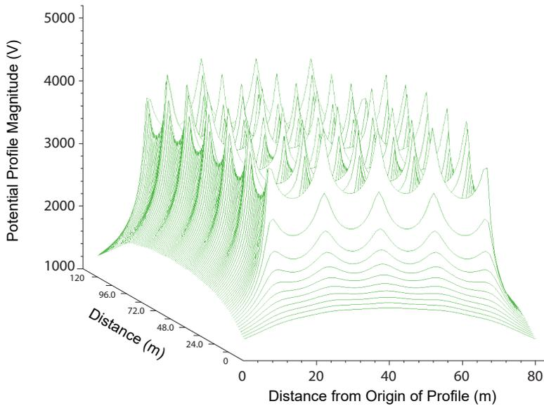
Figure 5-2: Potential contours of a ground grid
